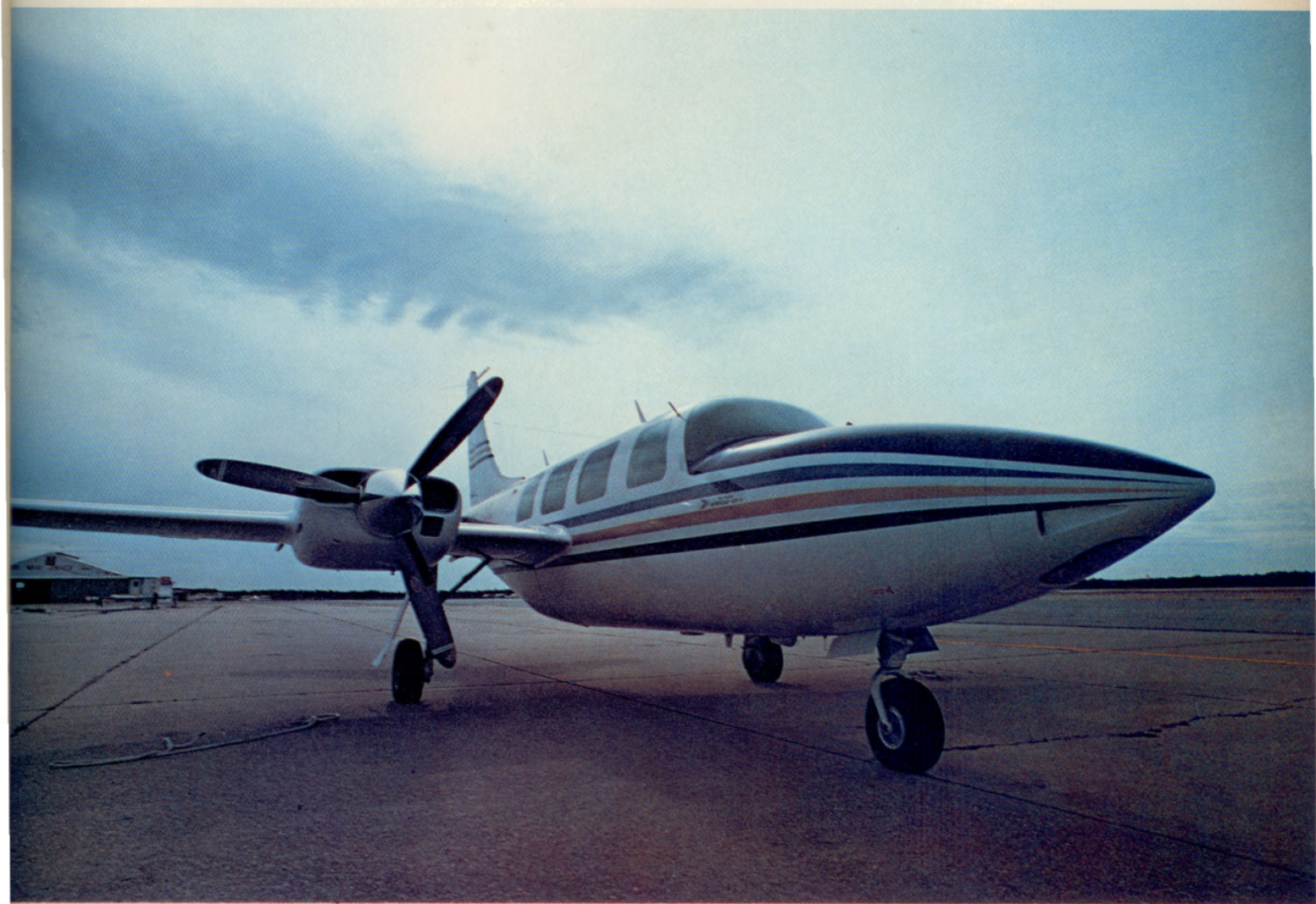
Shark-like snout and mid-fuselage wing offer a distinctive, clean profile to Ted Smith's Aerostar. Photos by the author.
